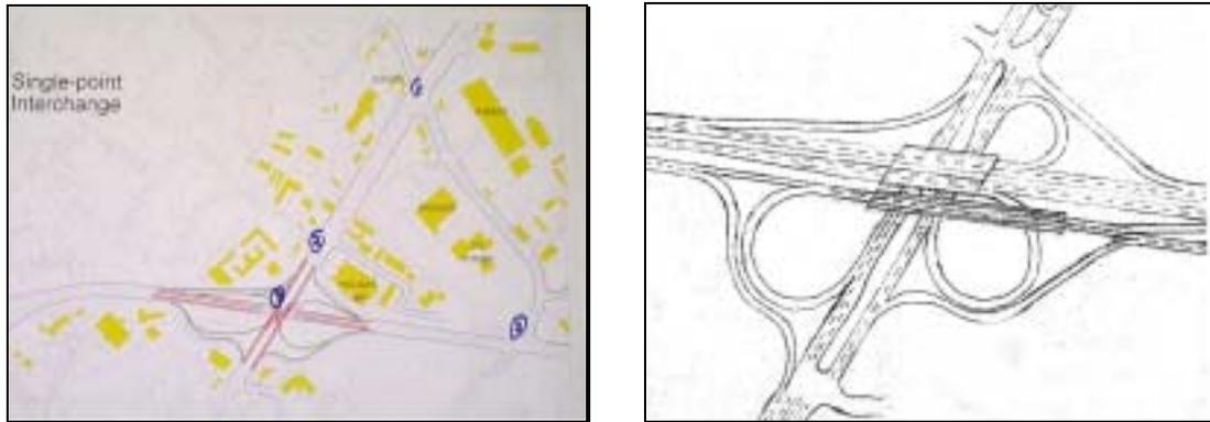
Figure 15 5) Single Point Urban Interchange; 6) Collector-distributor road concept
