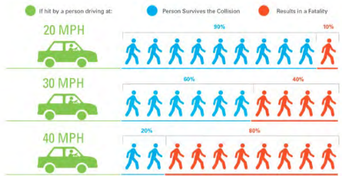
Figure 6. Demonstration of safety outcomes for pedestrians involved in crashes at different vehicle speeds. Taken from the Institute of Transportation Engineers .
